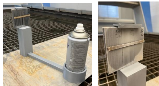
Figure 1. Preparation from the FDM 3D printing method, the distance between the nozzle and the samples is 250 mm
